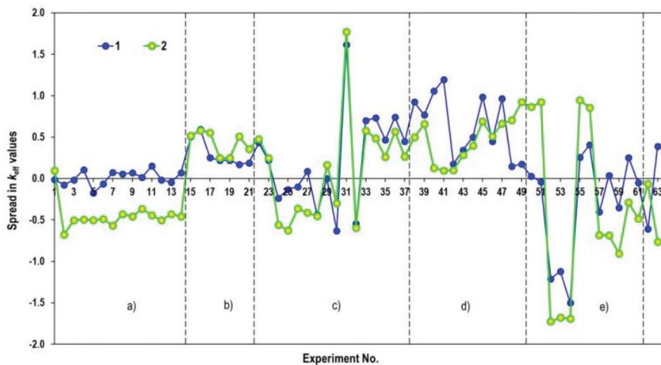
**Figure 1.** Deviations in calculated criticality values caused by the transition from the evaluated nuclear data library's older version to the new one: 1) magnitude  $(C^{\text{BNAB-93}}/C^{\text{BNAB-RF}} - 1)$  in percentage terms; 2) magnitude  $(C^{\text{ENDF/B-V}}/C^{\text{ENDF/B-VIII}} - 1)$  in percentage terms. Regions shown by dashed lines: a) sodium cooled fast reactor; b) lead cooled fast reactor; c) fabrication of MOX fuel; d) waste disposal in sand; e) CNFC facilities.
