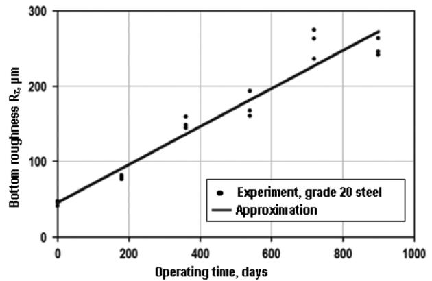
Figure 5. Turbine plant steam line bottom surface roughness as a function of operating time.
