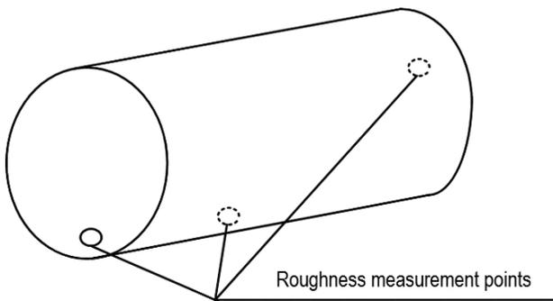
Figure 3. Pipe roughness measurement diagram.
