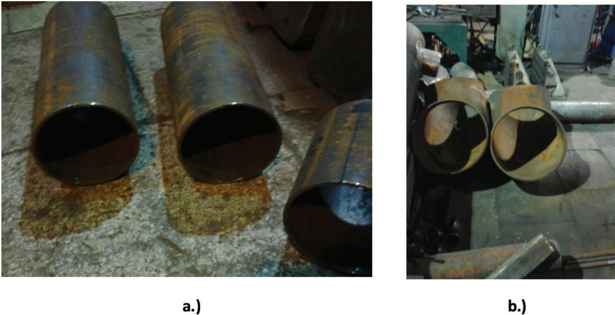
Figure 2. Defective pipe segments cut out of the NPP systems: a) 12Kh18N10T grade steel; b) grade 20 steel.
