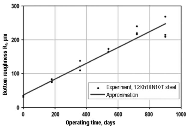
Figure 4. Bottom surface roughness of a high-pressure re-heater's piping as a function of operating time.
