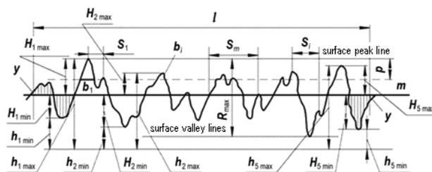
Figure 1. Schematic representation of the surface microrelief.
