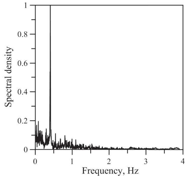
**Figure 6.** Normalized spectral density of temperature pulsations.
