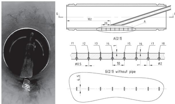
**Figure 2.** Location of the thermocouples on the MMTP.
