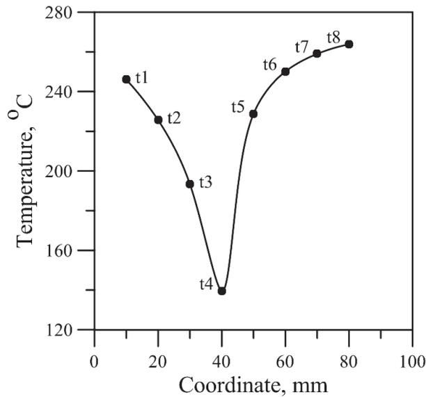
**Figure 4.** Averaged temperature profile in the coolant flow mixing zone.
