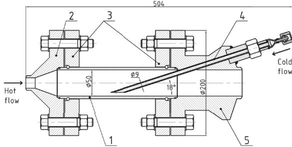
**Figure 1.** Experimental site 1. Experimental model; 2. Guide flange; 3. Cap flanges; 4. Peripheral tube; 5. Flange.
