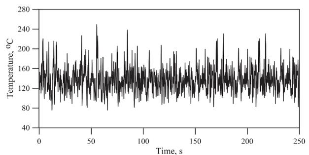
**Figure 3.** Experimental realization of the temperature-time dependence in the mixing zone.
