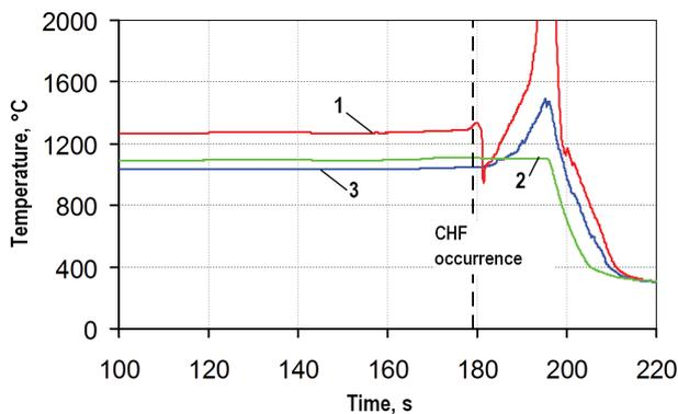
**Figure 4.** The temperature in the center of the fuel element kernel at the final stage of heating (the 0 s mark corresponds to a time of 12 h 41 min 32 s in the graph of Fig. 3): 1. TC  $T_1$  readings; 2. TC  $T_2$  readings; 3. TC  $T_3$  readings.
