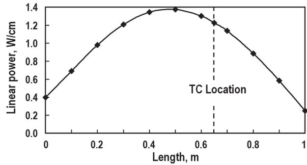
Figure 2. Axial active part linear power distribution.
