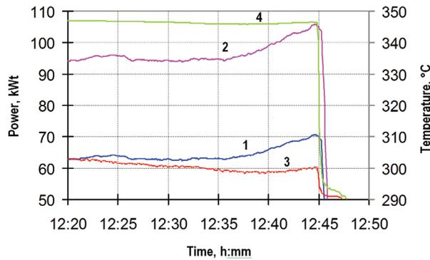
**Figure 3.** The dynamics of the EFA/experimental channel power and the coolant temperature: 1. EFA power; 2. experimental channel power; coolant temperature: 3. at the EFA inlet; 4. in the EFA inside; 5. at the EFA outlet.
