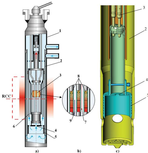
**Figure 1.** Experimental device: a) overall view; b) cross section in the reactor core center (RCC); c) coolant flow separation node; 1. channel shroud; 2. coolant flow separator; 3. fuel elements; 4. hole; 5. labyrinth seal; 6. cavity with a stagnant aqueous medium; 7. thermocouple (TC) in the coolant; 8. TC ( $T_1$ ,  $T_2$ ,  $T_3$  respectively) in the fuel kernel center; 9. direct charge detector (DCD).
