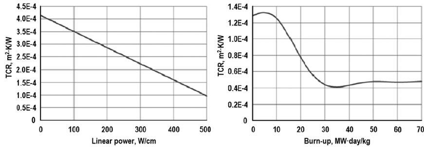
**Figure 2.** Fuel gap TCR s as a function of linear power for fresh fuel (based on chief engineer’s data) and of burn-up at linear power 448 W/cm (based on the Bushehr NPP final safety report data)
