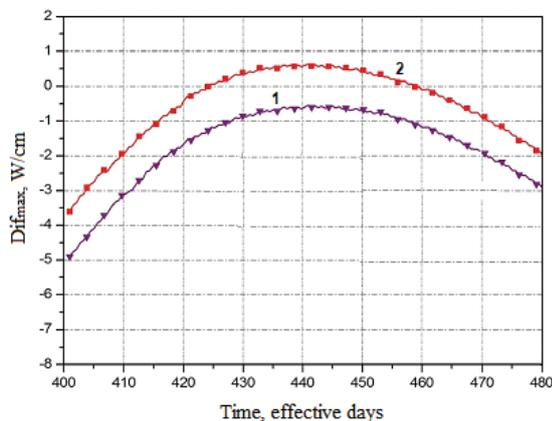
**Figure 5.** The maximum difference between the calculated and the maximum allowable linear power on the fuel element of the VVER-1000 at the end of the cycle for stationary fuel loading: 1 – Gap Conductance Coefficient without taking into account the dependence on burn-up; 2 – Gap Conductance Coefficient taking into account the dependence on burn-up
