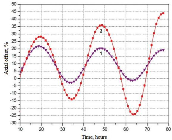
**Figure 7.** Axial offset as a function of time for stationary fuel loading of the VVER-1000 at 75 % of nominal power: 1 – Gap Conductance Coefficient without taking into account the dependence on burn-up; 2 – Gap Conductance Coefficient taking into account the dependence on burn-up
