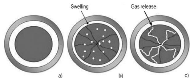
**Figure 1.** Variation in the cladding – fuel pellet gap width at high specific power  $Q_L > 400$  W/cm, for a PWR reactor: a) – fresh fuel; b) – fuel with burn-up; c) – high burn-up fuel
