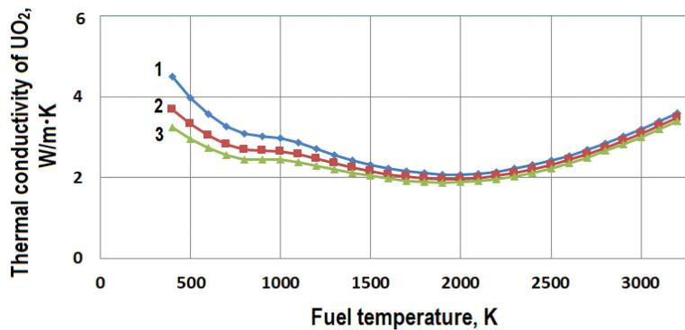
**Figure 3.** Thermal conductivity coefficient of  $UO_2$  as a function of temperature at different burn-up values: 1 – 20 MW·day/kg U; 2 – 40 MW·day/kg U; 3 – 60 MW·day/kg U
