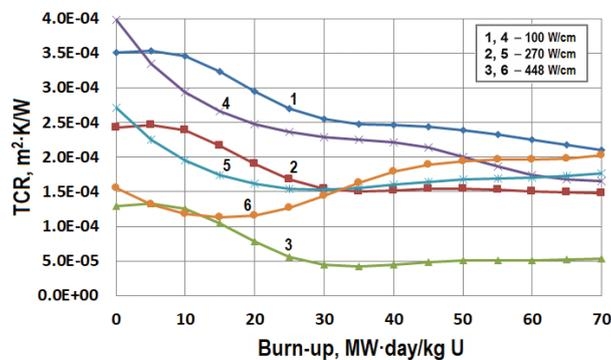
**Figure 4.** Gap TCRs as a function of fuel burn-up at different levels of linear power on fuel elements in VVER-1000 (semi-empiric dependences 1, 2, 3) and in PWR-1000 (Western dependences 4, 5, 6)
