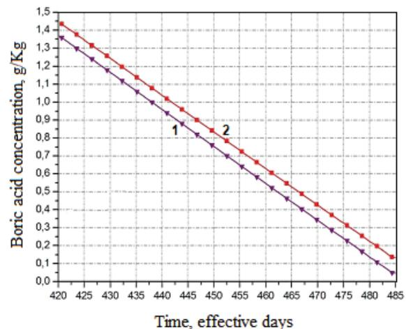
**Figure 6.** Dependence of boric acid concentration on the operating time of stationary fuel loading of the VVER-1000 at the end of the cycle: 1 – Gap Conductance Coefficient without taking into account the dependence on burn-up; 2 – Gap Conductance Coefficient taking into account the dependence on burn-up
