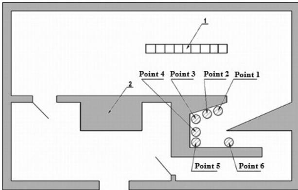
**Figure 5.** Arrangement of measurement points in the experimental study of different detectors in the field of background gamma radiation: 1. GU-200M irradiator; 2. Operator's position.
