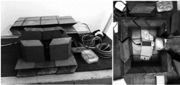
**Figure 2.** Detector based on CdZnTe inside the lead shielding.
