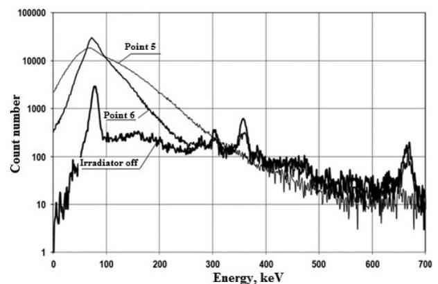
**Figure 8.** Test source spectra obtained at various points in the maze (compressed xenon ionization chamber detector).
