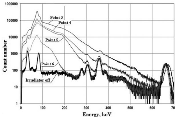
**Figure 7.** Test source spectra obtained at various points in the maze (LaBr<sub>3</sub> detector).
