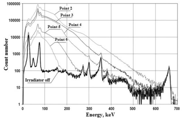
**Figure 6.** Test source spectra obtained at various points in the maze (CdZnTe detector).
