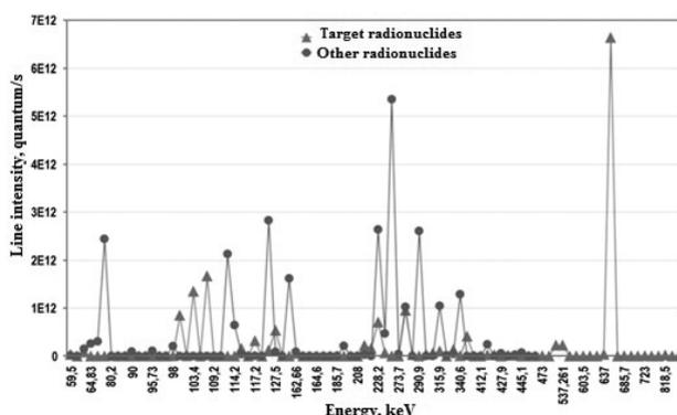
**Figure 1.** Theoretical  $\gamma$ -radiation spectrum of the measurement object with divided target and other nuclides.
