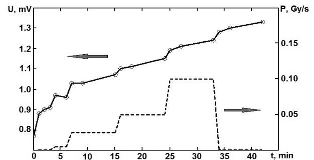
**Figure 1.** Time-dependences of the absorbed dose rate on the neutron source  $P$  and voltage  $U$  between the plates of a symmetrical supercapacitor.
