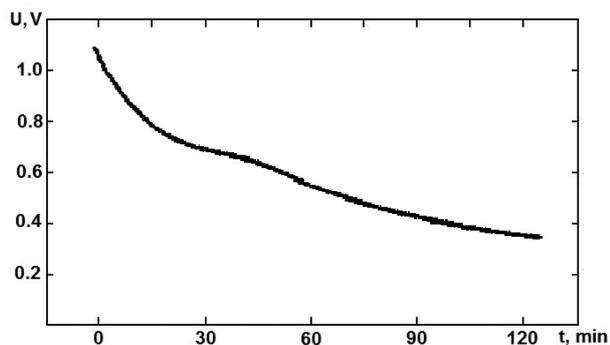
**Figure 3.** Changes in the electrical voltage between the asymmetrical supercapacitor plates the day after irradiation. The beginning of measurements corresponds to  $t = 0$ .
