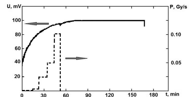
**Figure 2.** Time-dependences of the absorbed dose rate on the neutron source  $P$  and voltage  $U$  between the plates of an asymmetrical supercapacitor.
