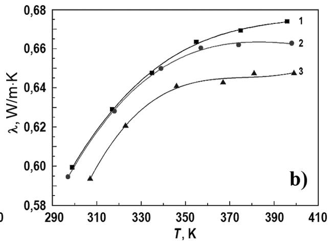
**Figure 5.** Dependence of thermal conductivity of aqueous solutions of boric acid on temperature and pressure: a)–0.1 MPa; б)–10 MPa. Concentration of boric acid: 1–0% (H<sub>2</sub>O); 2–1%; 3–3%; 4–5%
