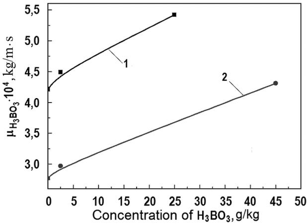
**Figure 3.** Dependence of viscosity of boric acid aqueous solutions on concentration at pressure equal to 0.1 MPa (Azizov and Ahundov 1996). Temperature: 1–65.6°C; 2–100°C
