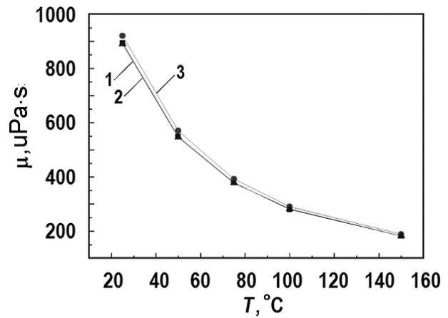
**Figure 4.** Dependence of viscosity of boric acid aqueous solutions on temperature for pressure equal to 1 MPa. Boric acid concentrations: 1–0 g/kg (H<sub>2</sub>O); 2–2 g/kg; 3–20 g/kg
