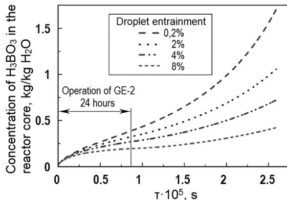
**Figure 7.** Variation of boric acid concentration in the reactor core at different values of droplet entrainment
