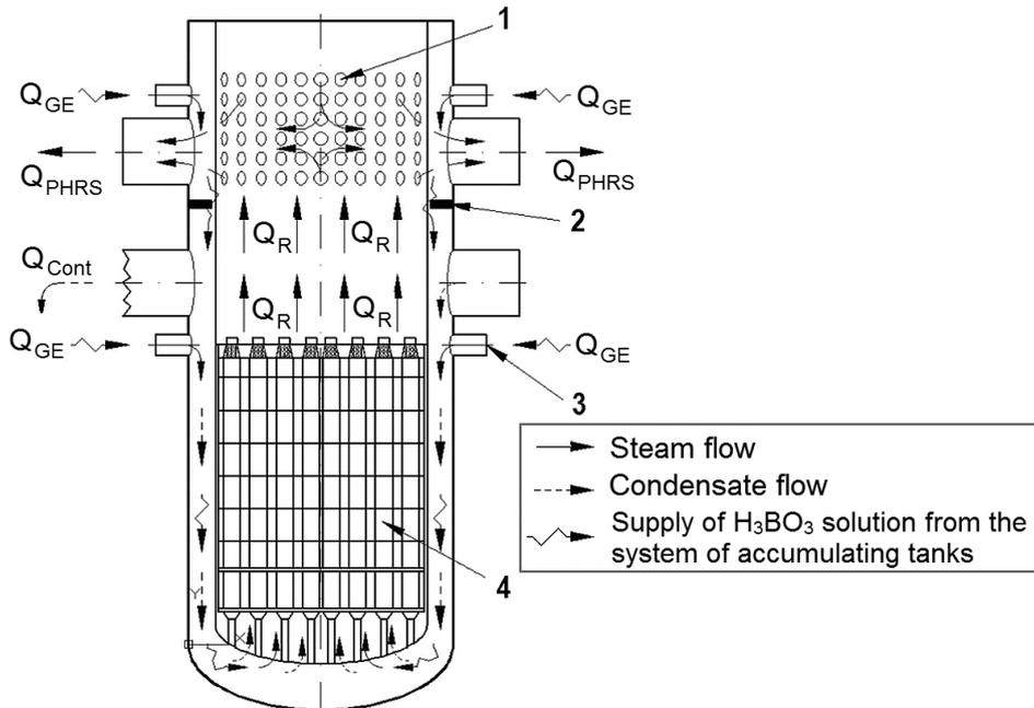
**Figure 6.** Mass transfer of boric acid in VVER reactor facility during accidents with rupture of the main coolant pipeline: 1 – reactor pit perforation; 2 – partitioning collar; 3 – flanged socket of the reactor core emergency cooling system; 4 – reactor core
