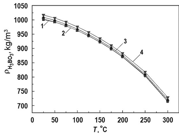
**Figure 1.** Dependence of density of boric acid solution on temperature at  $P = 10$  MPa. Boric acid concentrations: 1–0 g/kg ( $H_2O$ ); 2–3.1 g/kg; 3–18.6 g/kg; 4–43.4 g/kg
