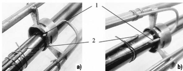
**Figure 2.** TET hot junction attachment points: a) – in the SG plane ; b) – 7 mm above the SG plane; TET forced against the SG cladding (1), TET forced against the cladding by means of wire binding (2)
