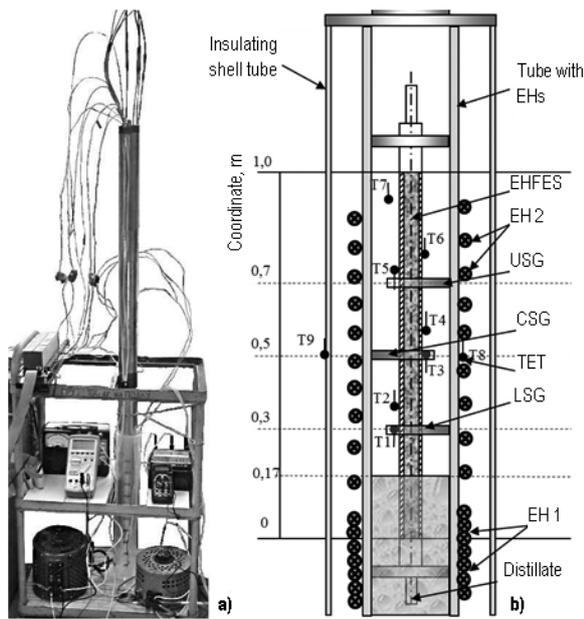
**Figure 1.** Laboratory facility: a) – overall view; b) – SG and TET arrangement in the LF
