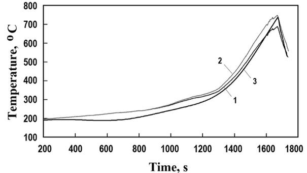
**Figure 5.** Time-temperature curve for experiment 2: TET readings (1); cladding temperature values determined using the TET readings with corrections taken into account (2); calculated cladding temperature values (3)
