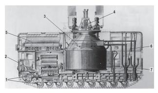
**Figure 4.** Scheme of the self-propelled vehicle with a reactor and service systems: 1. Self-propelled platform; 2. Body; 3. Reactor with shielding; 4. CPS actuators; 5. Radiator; 6. Pipeline of the primary circuit; 7. Technical water pipeline.
