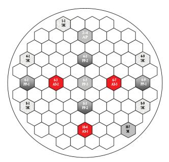
**Figure 1.** Layout of experimental channels for the <sup>99</sup>Mo production (ECs 4-1, 4-9, 8-1, and 8-9) in the VVR-ts reactor core (Website of JSC All-Regional Association Izotop).
