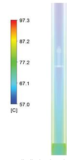
Figure 6. Temperature distribution through the coolant volume in the channel,  $^{\circ}$ C (90° rotated).
