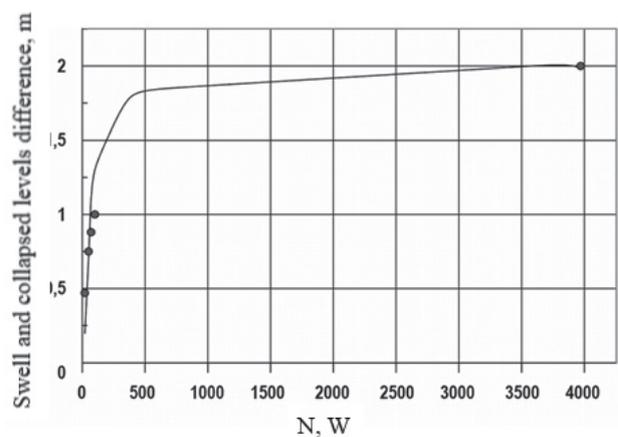
Figure 4. Calculation results as a function of the experimental data for  $\Delta H_{PM}$  with different fuel rod powers.
