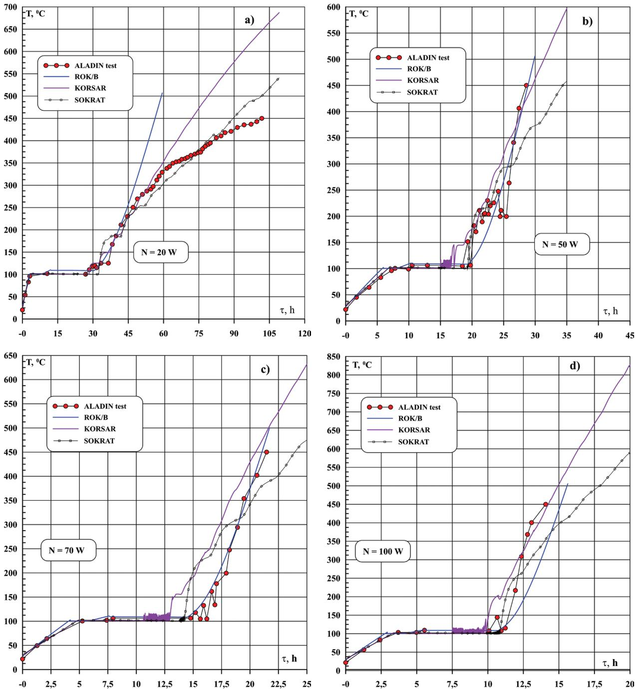
Figure 5. Cross verification results a. rod power 20 W; b. rod power 50 W; c. rod power 70 W; d. rod power 100 W (Partmann et al. 2018).
