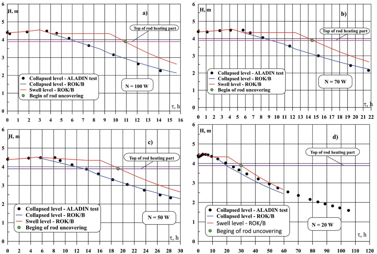
Figure 3. Compared experimental and calculated data of the coolant level dependence on time for different fuel rod powers.
