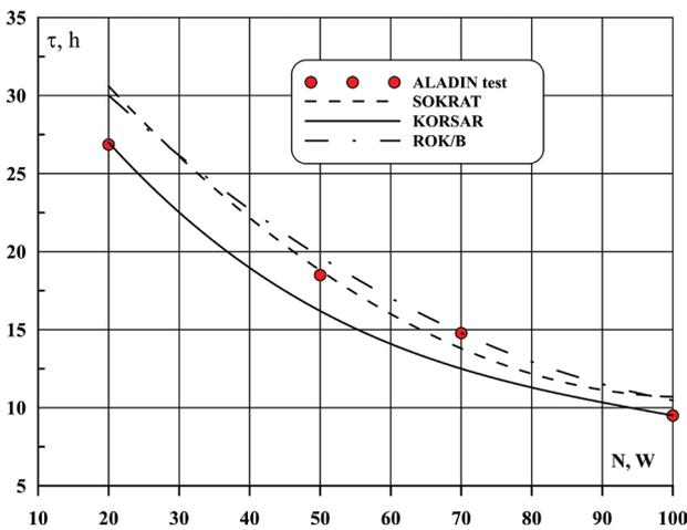
**Figure 6.** Results of the fuel surface uncovering onset time calculation (Partmann et al. 2018).
