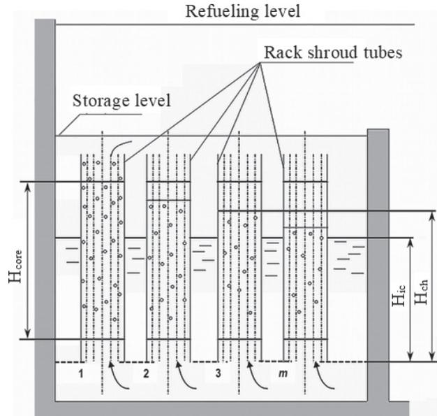
**Figure 1.** Overall view of the computational region with a single-tier SFA arrangement; 1, 2, 3, ...,  $m$  – numbers of groups of channels with assemblies.
