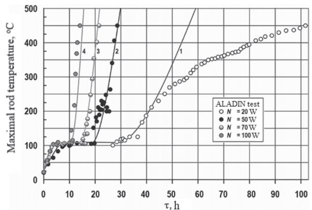
**Figure 2.** Experimental dependences of the maximum fuel temperature variation on time compared against the ROK/B calculations for different fuel rod powers: 1 –  $N_f = 20$  W; 2 –  $N_f = 50$  W; 3 –  $N_f = 70$  W; 4 –  $N_f = 100$  W.
