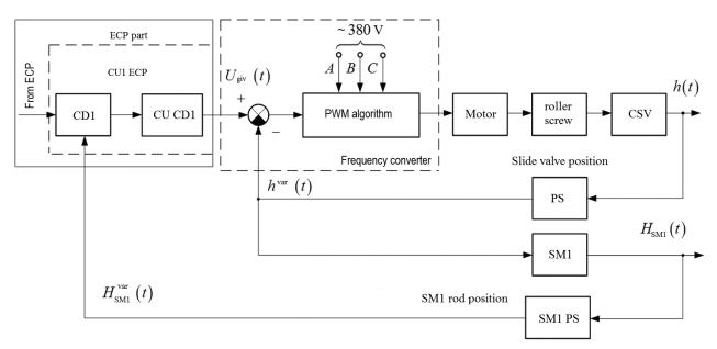
Figure 4. Functional diagram of the CU1 control unit with a control device (CU1 CD).
