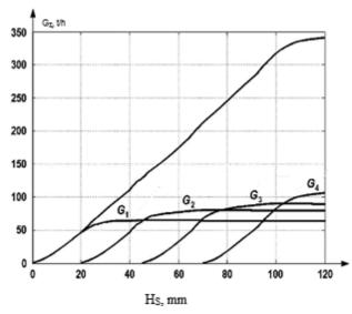
**Figure 6.** Diagrams of steam flows through the HPS control valves (SCV1 through SCV4) as a function of their strokes.
