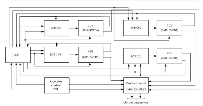
Figure 1. Functional diagram of the automatic control system for product T-63-13,0/0,25 (condensation mode).
