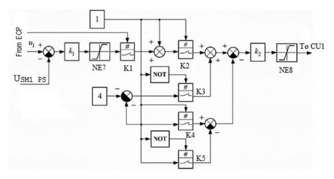
Figure 5. Block diagram of the control device for CU1 control unit.
