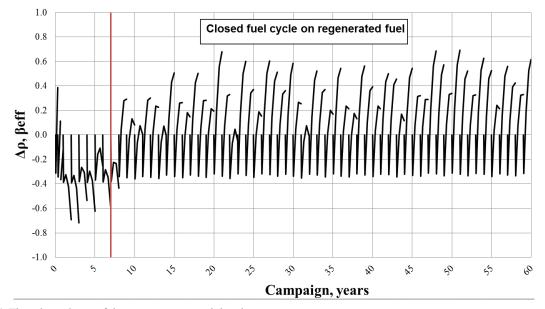
Figure 4. Time dependence of the reactor core reactivity change
