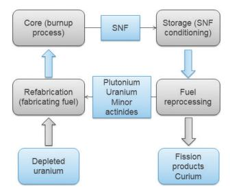
Figure 1. Diagram of the fuel cycle implementation in a leadcooled fast reactor
