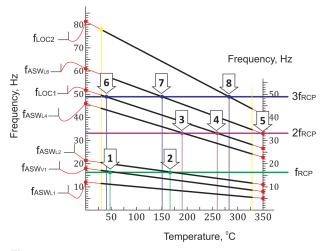
**Figure 7.** Dependence of the ASW central frequencies on the primary coolant temperature (digits 1 through 8 are the mode numbers).
