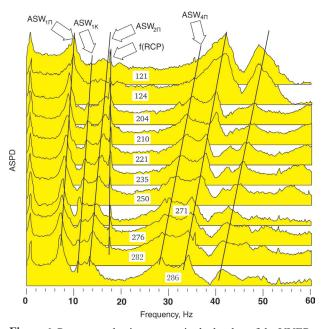
**Figure 6.** Pressure pulsation spectra in the hot leg of the VVER-1200 primary loop for a temperature range of 122 to 286 °C. ASW coalescence with the second harmonic of the RCP rotational frequency at 276 °C. Coalescences for lower- and higher-mode ASW at low temperatures.
