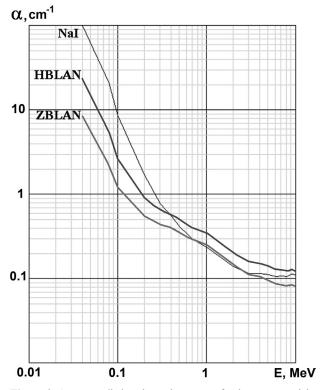
Figure 3. Gamma radiation absorption spectra for detector materials.
