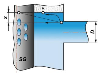
Figure 4. Scheme of bubble rise in the peripheral cavity.
