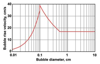
Figure 1. Dependence of the bubble rise velocity on its size.
