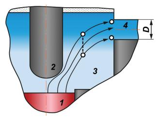
**Figure 3.** Scheme of bubbling up in the central cavity: 1) The core; 2) the CPS actuator column; 3) FR central cavity; 4) LC collector.
