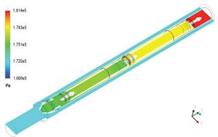
Figure 6. Circulation water pressure distribution in the channel's vertical cross-section.
