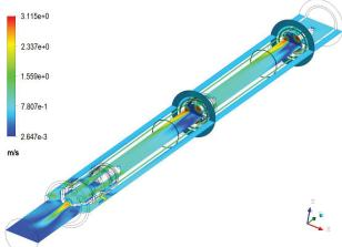
**Figure 7.** Circulation water velocity distribution in the channel's vertical cross-section.
