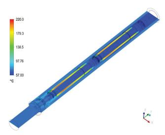
**Figure 4.** Temperature distribution in the vertical cross-section of the experimental channel.
