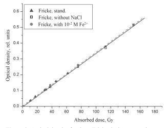
**Figure 2.** Optical density for three Fricke dosimeter versions as a function of the <sup>60</sup>Co gamma radiation dose.
