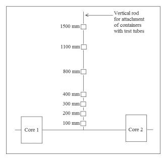
**Figure 1.** Irradiation geometry of chemical Fricke dosimeters at the BARS-6 reactor in pulsed and continuous modes.
