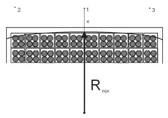
**Figure 4.** A model to assess the radiological situation around a hangar-type storage facility.
