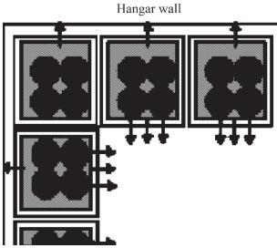
**Figure 3.** Diagram of the external cask orientation in the storage facility's peripheral rows.
