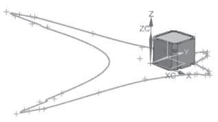
Figure 6. Software-predicted distribution of the gamma dose rate from a filled NZK-150-1,5P cask.
