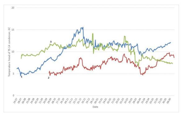
Figure 4. Temperature head change for the TS-14 condenser: 1 – temperature head in 2016–2017; 2 –temperature head in 2017–2018; 3 – temperature head in 2018–2019
