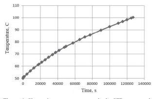
**Figure 4.** Change in water temperature in the SFP upon termination of forced circulation (compacted storage of SFAs without water loss in the SFP).
