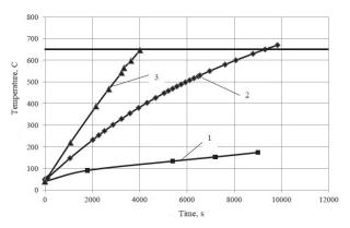
**Figure 7.** Changes in the SFA temperature in the emergency FA unloading compartment: 1 – decrease in the water level to the SFA heads; 2 – the SFAs exposed by 25%; 3 – the SFAs exposed by 50%.
