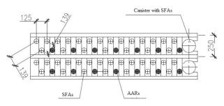
**Figure 1.** Layout of non-canister SFA placement in the SFP. AAR = additional absorber rods.
