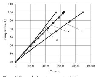
**Figure 6.** Changes in the water temperature in the emergency FA unloading compartment: 1 – decrease in the water level to the SFA heads; 2 – the SFAs exposed by 25%; 3 – the SFAs exposed by 50%.
