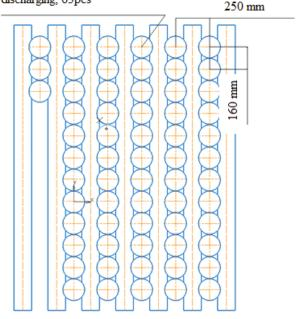
Figure 2. Layout of the emergency FA discharging compartment.
