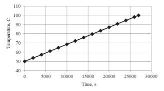
**Figure 5.** Water heating to the saturation temperature in the SFP (sealed FA storage, partial loss of water with 50% exposure of the SFAs).
