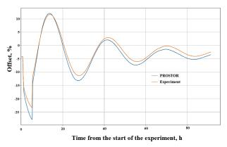
**Figure 1.** Results of modeling free xenon oscillations at a power equal to 75% of the rated value for the first campaign of Kalinin NPP-3. Axial offset behavior.
