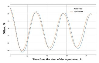
**Figure 2.** Results of modeling free xenon oscillations at a power equal to 75% of the rated value for the first campaign of Kalinin NPP-4. Axial offset behavior.
