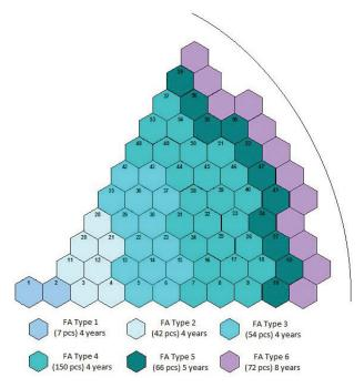
Figure 1. Reactor core map grid.
