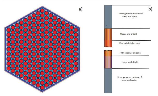
Figure 2. Fuel assembly calculation model: a) - horizontal projection; b) - vertical projection.
