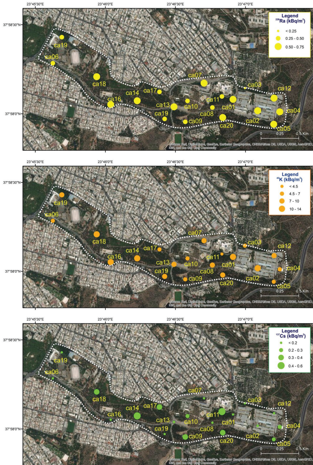
Figure 7. Radiological maps of ^{226}\text{Ra} (top), ^{40}\text{K} (middle) and ^{137}\text{Cs} (bottom).
