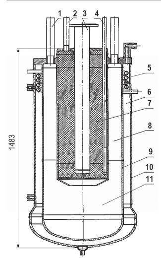
**Figure 2.** Design of the sodium impurity cold trap for the BR-10 reactor: 1 – sodium inlet nozzle; 2 – sodium outlet nozzle; 3 – heater cavity; 4 – thermocouple pocket; 5 – water cooling coil; 6 – toluene cavity; 7 – filter; 8 – sodium cooling channel; 9 – cold trap inner body; 10 – cold trap outer body; 11 – sump.
