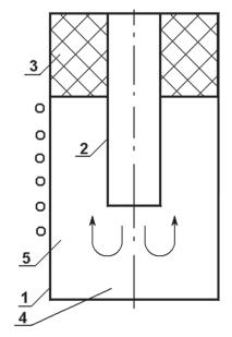
**Figure 1.** Cold trap schematic design: 1 – trap body; 2 – supply channel; 3 – filter; 4 – sump; 5 – cooling area.
