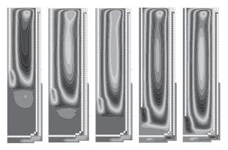
Figure 4. Pattern of the sodium flow in the cold trap with different downcomer lengths.
