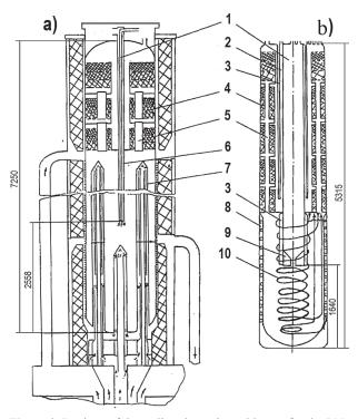
**Figure 3.** Designs of the sodium impurity cold traps for the BN-600 (a) and BN-350 (b) reactors: 1 – central tube; 2 – outside regenerator channel; 3 – air gap; 4 – filter; 5 – flow-through tubes; 7 – air cooling tubes; 8 – cooling jacket; 9 – cone; 10 – coil.
