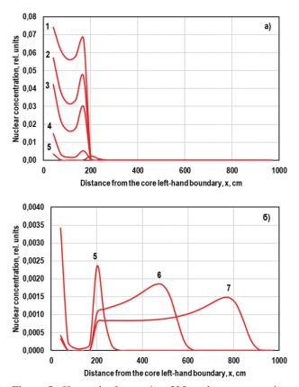
**Figure 5.** Change in the uranium-235 nuclear concentration lengthwise the core after 100 days (1), 200 days (2), 300 days (3), 500 days (4), 1000 days (5), 5000 days (6), and 9000 days (7): a) – seed region; b) – feed region.
