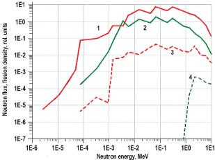
**Figure 6.** Neutron and fission density spectra at the fission wave formation start time: 1, 2 -flux spectra in the seed region area and in the adjacent breeding region (blanket) respectively; 3, 4 -fission density spectra in the seed region and in the blanket.
