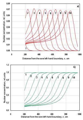
**Figure 3.** Change in the uranium-233 (a) and thorium-232 (b) nuclear concentration along the core after 100 days (1), 1000 days (2), 2000 days (3), 3000 days (4), 4000 days (5), 5000 days (6), 6000 days (7), 7000 days (8), 8000 days (9), and 9000 days (10).
