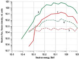
**Figure 7.** Neutron and fission density spectra after 2000 days from the reactor fission-wave operation start time: 1, 2 -flux spectra in the seed region area and in the blanket respectively; 3, 4 - fission density spectra in the seed region and in the blanket.
