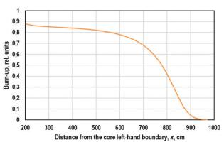
Figure 8. Fuel burn-up lengthwise the core after 9000 days.
