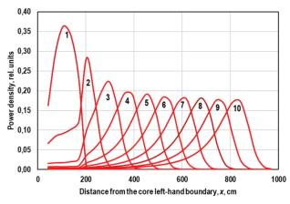
**Figure 2.** Power density distribution along the core after 100 days (1), 1000 days (2), 2000 days (3), 3000 days (4), 4000 days (5), 5000 days (6), 6000 days (7), 7000 days (8), 8000 days (9), and 9000 days (10).
