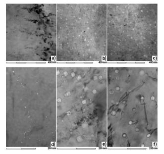
Figure 1. Vacancy pores in the samples after irradiation during 22 years (a,b,c) and 33 years (d,e,f) to damaging doses of ~1 dpa ate temperature of ~370 °C (a,d), to damaging doses of ~16 dpa (b) and ~33 dpa (f) at temperature of ~415 °C, to damaging dose of ~21 dpa (c) at ~425 °C and to damaging dose of ~24 dpa (f) at ~430 °C.
