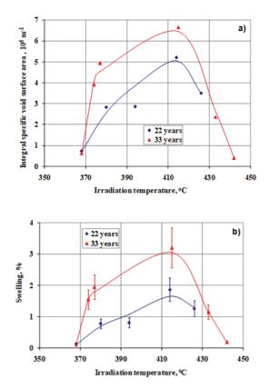
**Figure 4.** Temperature dependences of integral specific void surface area (a) and swelling (b) for large-size voids in Cr18Ni9 steel after irradiation in the BN-600 reactor during 22 years and 33 years.
