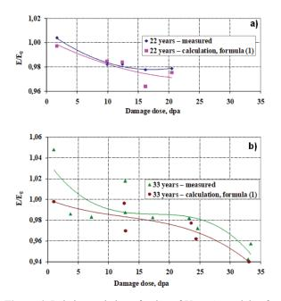
**Figure 6.** Relative variation of value of Young's modulus for Cr18NIi9 steel after irradiation in the BN-600 reactor during 22 years and 33 years (a.b) and the value of Young's modulus theoretically calculated according to the formula (1) using the value of swelling of samples depending on the damagie dose.
