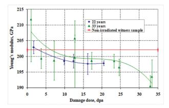
**Figure 5.** Variation of Young's modulus for Cr18Ni9 steel after irradiation in the BN-600 reactor during 22 years and 33 years depending on the damage radiation dose.
