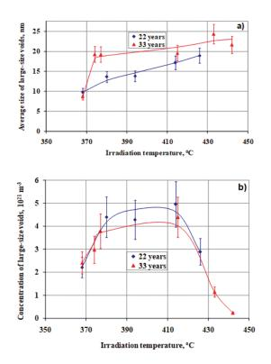
**Figure 3.** Temperature dependences of the average pore size (a) and concentration (b) of large-size pores in Cr18Ni9 steel after irradiation in the BN-600 reactor during 22 years and 33 years.
