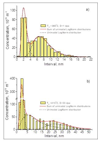
**Figure 2.** Histograms of void distributions according to void sizes for samples irradiated at  $\sim$ 370 °C to damage dose >1 dpa (a) and at  $\sim$ 415 °C to damage dose of  $\sim$ 33 dpa (b).
