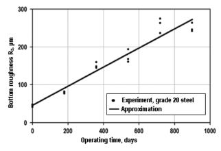
**Figure 5.** Turbine plant steam line bottom surface roughness as a function of operating time.
