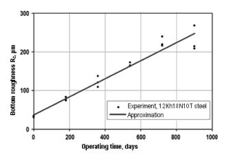
**Figure 4.** Bottom surface roughness of a high-pressure reheater's piping as a function of operating time.
