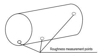
Figure 3. Pipe roughness measurement diagram.
