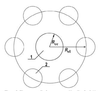
**Figure 3.** Elementary cell of reactor core with radius  $R_{\rm el}$ =2,46 cm for the determination of temperature field: 1 – coolant channel  $R_{\rm cc}$  = 1.05 cm; 2 – nuclear fuel channel  $R_{\rm nf}$  = 0.63 cm
