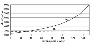
Figure 2. Dependences of fluxes of thermal  $\Phi_t$  and damaging  $\Phi_d$  neutrons on the nuclear fuel burnup
