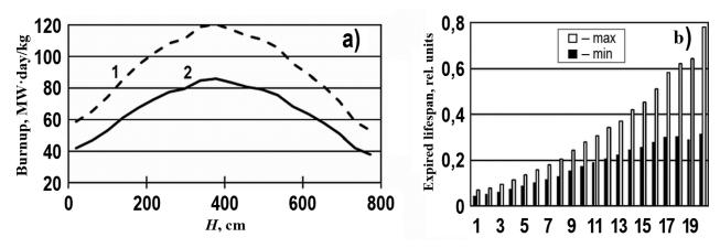
**Figure 6.** a). Dependence of burnup depth along the core height for fuel block at the end of nuclear fuel irradiation micro-campaign:  $1 - \max_{r} (1.23)$ ;  $2 - \min_{r} k_{r} (0.88)$ . b). Expired lifespan of graphite at the end of nuclear fuel irradiation campaign for sections of fuel blocks with maximum (1.23) and minimum (0.88)  $k_{r}$
