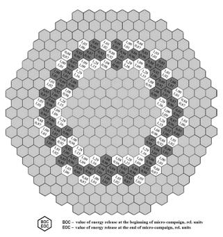
**Figure 5.** Map of GT-MHR reactor core: white – fuel assemblies after irradiation during the burnup cycle; gray – fresh fuel assemblies; graphite reflector at the periphery and in the center
