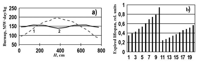
**Figure 8.** a). Dependence of burnup depth on the height of the reactor core at the end of nuclear fuel irradiation campaign: 1 -without taking re-shuffling of graphite blocks into account; 2 -taking re-shuffling of graphite blocks into account. b). Dependence of the value of expired lifespan of graphite along the core height at the end of reactor fuel irradiation campaign with different non-uniformity of heat release after re-shuffling the blocks at the middle of fuel irradiation campaign
