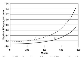
**Figure 4.** Time dependence of the expired lifespan of graphite along the core height: 1 – nuclear fuel residence time equal to 1090 eff. days; 2 – time between fuel re-shuffling in the core equal to 545 eff. days
