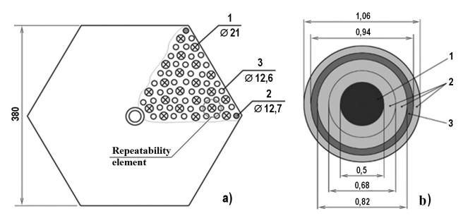
**Figure 1.** a). Fuel block of GT-MHR reactor core: 1 – channel for coolant passage; 2 – channel for burnable neutron absorber; 3 – fuel channel. b). Design of fuel microelement: 1 – uranium dioxide; 2 – pyrolytic graphite; 3 – silicon carbide.
