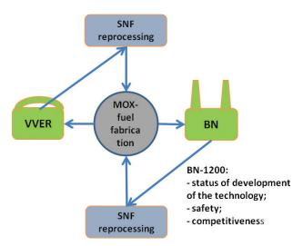
Figure 1. Layout of mutual fuel support of VVER and BN.
