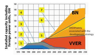
**Figure 2.** Proportion between BN and VVER reactors in the two-component nuclear power generating system: 1 – VVER-440; 2 – RBMK; 3 – VVER-1000; 4 – BN-600; 5 – BN-800; 6 – VVER-TOI; 7 – BN-1200.
