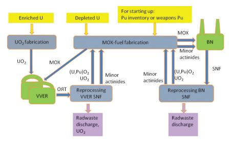
Figure 4. Layout of centralized (distributed over separate sites) NFC within two-component nuclear power generating system.
