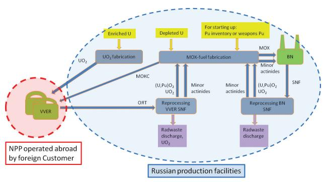
Figure 5. Organization of operation of two-component nuclear power generating system with closed nuclear fuel cycle with participation of foreign customers.
