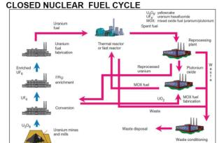
In the closed' fuel cycle the spent fuel is reprocessed and the residual uranium and plutonium are separated from the wast products. Both the uranium and the plutonium can be recycled into new fuel elements for use in thermal and fast reactors.
