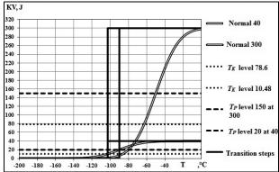
**Figure 2.** Comparison of  $T_K$  and  $T_p$  during testing standard-size  $(KV = 300 \text{ J/cm}^2)$  and small-size  $(KV = 40 \text{ J/cm}^2)$  samples for mechanical testing KStK1 brittle fracture resistance.
