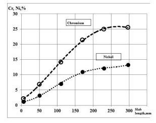
**Figure 4.** Distribution of chromium and nickel along the length of the process model of the weld boundary between base metal and the anticorrosive cladding metal in the state without additional melting down.
