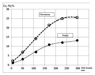
**Figure 5.** Distribution of chromium and nickel along the length of the process model of the weld boundary between base metal and the anticorrosive cladding metal after additional equalizing melting down.
