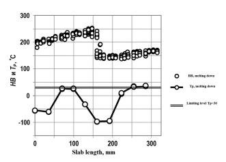
**Figure 6.** Distributions of hardness *HB* after additional equalizing melting down and  $T_p$  after melting down along the length of the process model of the weld fusion boundary between the base metal and the anticorrosive cladding metal before and after equalizing melting down.
