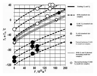
**Figure 1.** Dose-time relationships of  $T_{\kappa}$  and  $T_{p}$  for the results of testing standard-size and small-size samples made of KStK1 with base chemical composition subjected to "thermal hardening" treatment.
