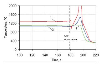
**Figure 4.** The temperature in the center of the fuel element kernel at the final stage of heating (the 0 s mark corresponds to a time of 12 h 41 min 32 s in the graph of Fig. 3): 1. TC  $T_1$  readings; 2. TC  $T_2$ , readings; 3. TC  $T_3$  readings.
