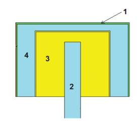
**Figure 2.** Cross-section of the detector's detection unit model: 1 – aluminum lid with a carbon window; 2 – wire leading channel to detector crystal; 3 – detector crystal; 4 – vacuum gap
