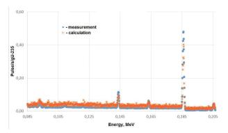
**Figure 4.** Comparison of the measured and calculated gamma quanta spectra from cellulose-containing cask. The waste material density is 0.708 g/cm<sup>3</sup>
