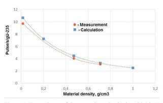
**Figure 5.** Dependence of the count intensity in the 185.7 keV peak on the density of the waste material in the form of cellulose with a small content of uranium ( $\sim 1 \text{ g of }^{235}\text{U}$ )
