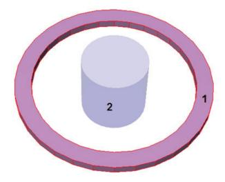
**Figure 3.** Computational geometry in modeling of spectra from waste-containing casks: 1 – ring-shaped detector with a lead collimator; 2 – cask with waste
