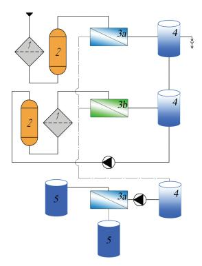
**Figure 1.** Schematic diagram of the facility: 1 – microfilter; 2 – salt dissolver 3a – hyperfiltration apparatus; 3b – hyperfiltration (nanofiltration) apparatus; 4 – intermediate tank; 5 – control tank.
