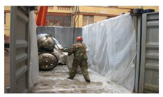
**Figure 7.** Loading of the large-sized radiation-contaminated equipment into the PU-2ETS-ST transport containers.
