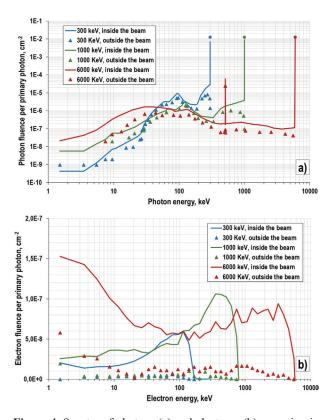
**Figure 4.** Spectra of photons (a) and electrons (b) emerging in the water at the depth of 5 cm from the monoenergetic photon source. Black circles in Figure (a) indicate initial fluences of the sources (photon fluences at the depth of 0 cm).
