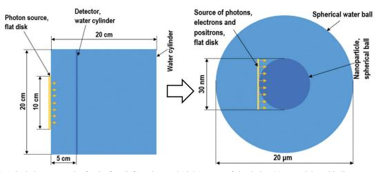
Figure 2. Calculation geometries for the first (left) and second (right) stages of simulation. Nanoparticles with diameters equal to 2 nm and 30 nm were simulated during the second stage.
