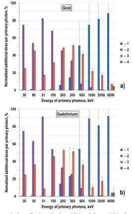
**Figure 6.** Contributions in the additional dose within the area from the surface to 100 nm from the center of nanoparticles of gold and gadolinium with  $\phi$  30 nm positioned inside the beam from electrons, primary photons, secondary photons and positrons: 1 – electrons; 2 – primary photons; 3 – secondary photons; 4 – positrons. Statistical uncertainties are indicated with bars.
