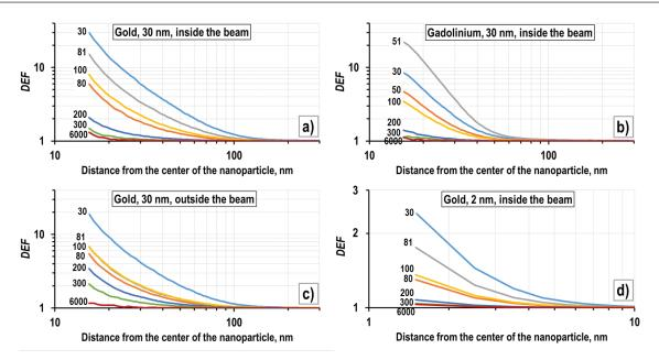
**Figure 5.** Radial *DEF* for nanoparticles: a) – Au  $\phi$  30 nm, inside the beam; b) – Gd  $\phi$  30 nm, inside the beam; c) – Au  $\phi$  30 nm, outside the beam; d) – Au  $\phi$  2 nm, inside the beam. Figures near the curves indicate energies of primary photons in keV. Curves for 81 keV and 100°keV in Fig. c) practically coincide.
