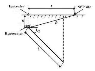
**Figure 2.** Calculated schematics of deep-focus earthquake: *h* is the hypocenter depth, km; *L* is the fault line length, km;  $\alpha$  is the incidence angle, degrees; *r* is the distance to the NPP, km; *R* is the hypocentral distance to the NPP, km
