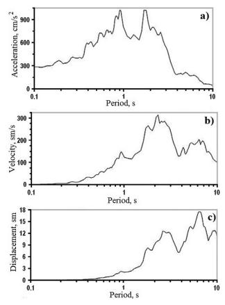
**Figure 5.** Response accelogram (a), velocitogram (b) and displacement diagram (c) on the NPP site (damping coefficient is equal to 5%)
