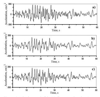
**Figure 4.** Seismic record of the Madhupur earthquake: a) – surface; b) – base; c) – rock exposure
