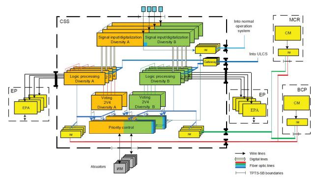
**Figure 1.** Integrated TPTS-SB-based CSS: EP – emergency protection; MCR – main control room; BCP – backup control panel; ULCS – upper level control system; CSS – control safety system; EPA – emergency protection automatics; IM – interface module; CM – communication module.
