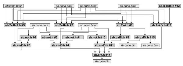
Figure 3. Mathematical model graph corresponding to the functional diagram in Fig. 2 The vertices *sb.conn.bout* correspond to the input signals of the functional diagram, the vertices *sb.conn.bin* correspond to the output signals. The remaining vertices correspond to the functional blocks and have a sequence number.
