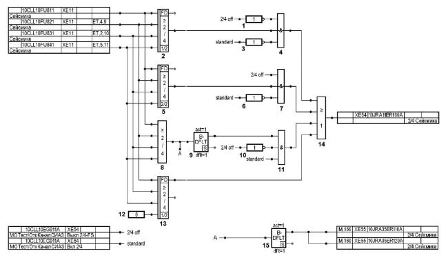
Figure 2. Functional diagram of processing signals from seismic sensors.
