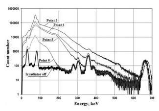
**Figure 7.** Test source spectra obtained at various points in the maze (LaBr, detector).
