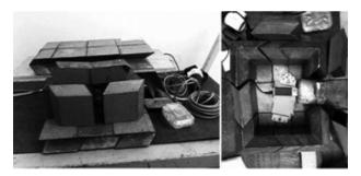
Figure 2. Detector based on CdZnTe inside the lead shielding.
