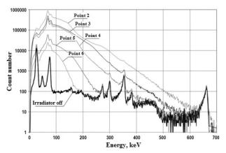
Figure 6. Test source spectra obtained at various points in the maze (CdZnTe detector).
