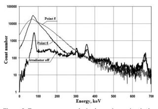
Figure 8. Test source spectra obtained at various points in the maze (compressed xenon ionization chamber detector).
