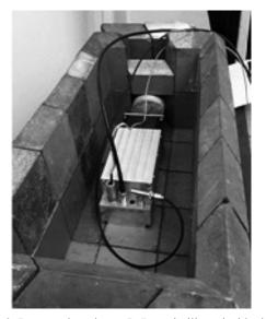
**Figure 3.** Detector based on a LaBr<sub>3</sub> scintillator inside the lead shielding.
