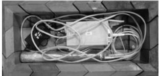
Figure 4. Detector based on an ionization chamber with compressed xenon inside the lead shielding.
