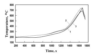
Figure 5. Time-temperature curve for experiment 2: TET readings (1); cladding temperature values determined using the TET readings with corrections taken into account (2); calculated cladding temperature values (3)
