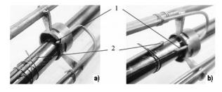
Figure 2. TET hot junction attachment points: a) – in the SG plane; b) – 7 mm above the SG plane; TET forced against the SG cladding (1), TET forced against the cladding by means of wire binding (2)
