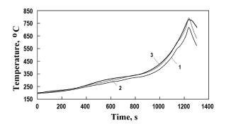
**Figure 4.** Time-temperature curve for experiment 1: TET readings (1); cladding temperature values determined using the TET readings with corrections taken into account (2); calculated cladding temperature values (3)
