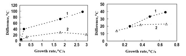
**Figure 3.** Variation of the difference in the TET readings for  $T_4 - T_3$ ,  $T_6 - T_5$  as a function of the rate of growth in the TET readings in the CSG (1) and in the LSG (2) at 300°C (a) and 600°C (b)
