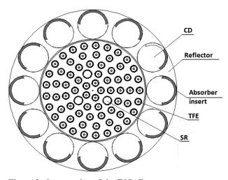
Figure 2. Cross-section of the TOPAZ-type converter reactor (Yarygin et al. 2016)
