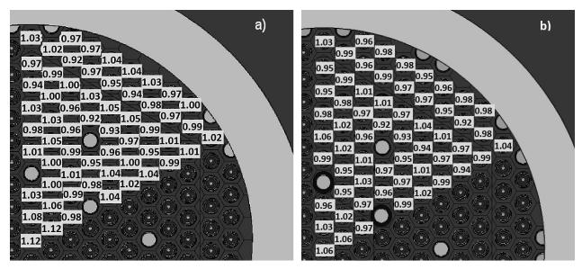
Figure 5. Power density distribution by fuel elements with the core split into two (a) and three (b) sections
