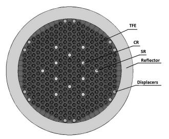
Figure 4. The core of a water-moderated water-cooled TCR
