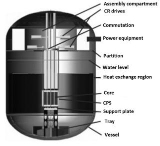
Figure 1. Conceptual design of an NPP based on a thermionic NPS
