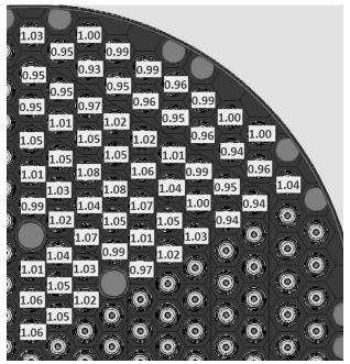
**Figure 7.** Power density distribution by fuel elements with the core split into four sections
