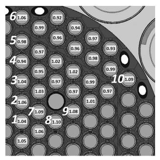
Figure 8. Power density distribution by fuel elements with the core split into three sections
