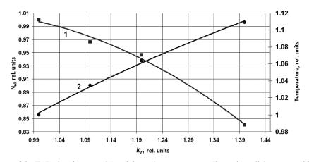
Figure 3. Dependence of the TCR electric power (1) and the emitter temperature (2) on the radial power peaking factor
