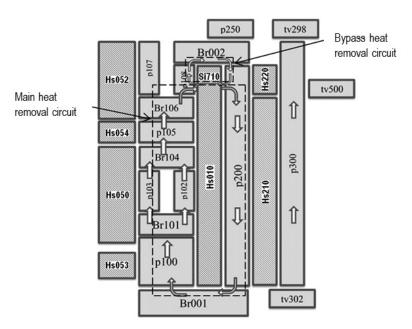
Figrue 2. Ampoule channel and downcomer nodalization pattern
