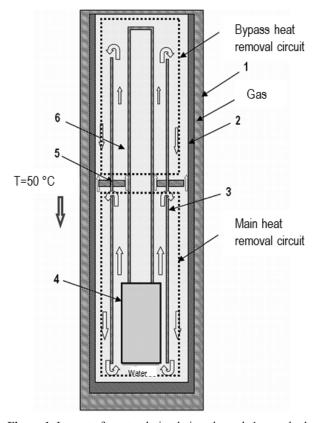
**Figure 1.** Layout of a natural-circulation channel: 1 outer body 2 inner body 3 separator 4 dummy holder with samples 5 flow limiter 6 bar
