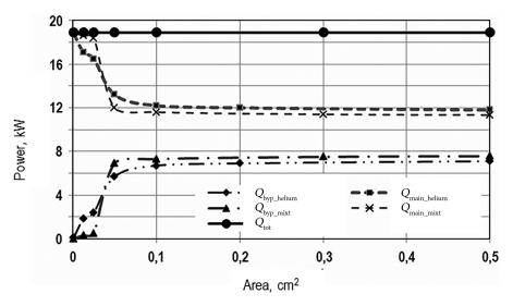
Figure 3. Total power  $(\mathbf{Q}_{tot})$ , main circulation circuit power  $(\mathbf{Q}_{main})$  and bypass power  $(\mathbf{Q}_{byp})$  as functions of the flow limiter orifice area
