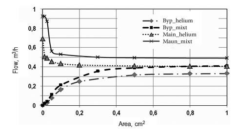
Figure 5. Bypass and main flow rates as functions of the flow limiter orifice area
