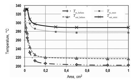
Figure 4. Sample inlet and outlet temperatures as functions of the flow limiter passage area
