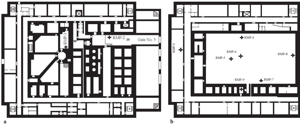
**Figure 6.** Positions of the radiation monitoring points inside the reactor building: **a.** Elevation +0.0 m; **b.** Elevations +8.4 m and 13.2 m.
