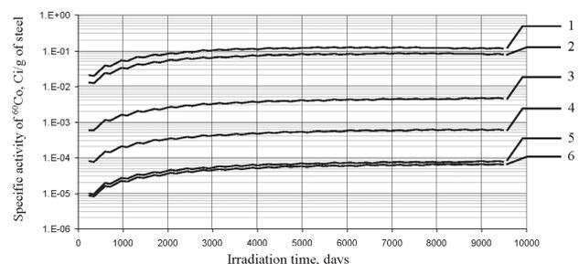
**Figure 5.** Induced activity of  $^{60}\text{Co}$  in the reactor core structural components as a function of irradiation time: 1 – lower end parts of beryllium blocks; 2 – upper support plate; 3 – vessel between elevations of -200 and 200 from the core mid position; 4 – vessel outside elevations of -200 and 200 from the core mid position; 5 – lower end parts of beryllium blocks; 6 – bottom shell.
