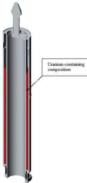
**Figure 1.** Design of a target with direct-flow cooling for  $^{99}\text{Mo}$  production.
