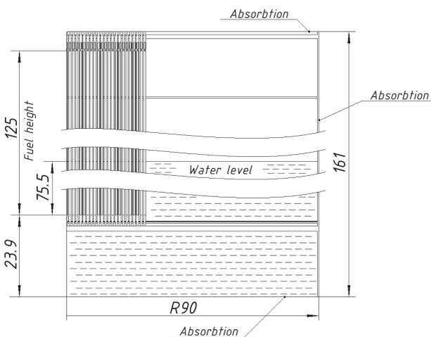
**Figure 3.** Vertical cross-section of the ZR-6 computational model.
