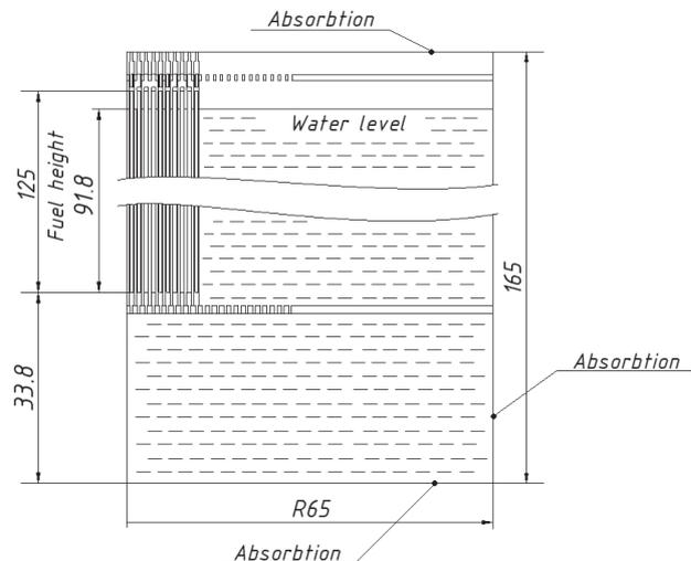
**Figure 1.** Vertical cross-section of the Stend P computational model.
