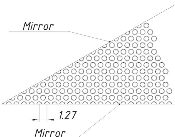
**Figure 4.** Horizontal cross-section of the ZR-6 computational model.
