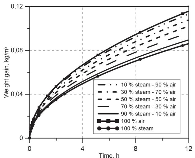
**Figure 2.** Weight gain behavior for oxidation in mixtures with different steam and air ratios at 800 °C.
