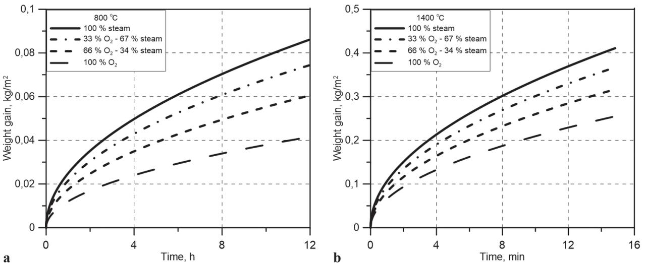
Figure 4. Weight gain behavior for oxidation in mixtures with different steam and oxygen ratios at a. 800 °C and b. 1400 °C.
