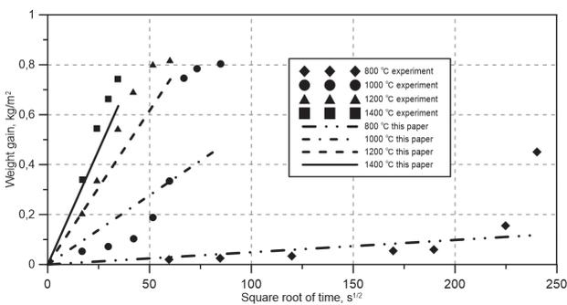
**Figure 1.** Simulation results versus experimental data Steinbrück 2009 for oxidation in a mixture of steam and air in a ratio of 50% to 50% (vol.).
