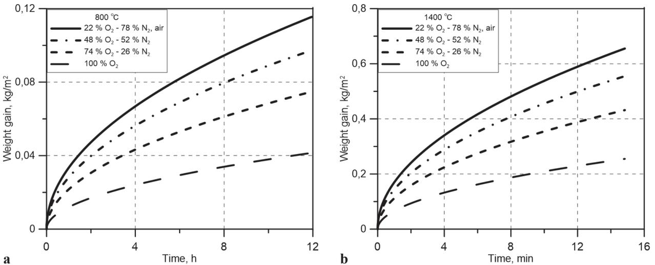
Figure 3. Weight gain behavior for oxidation in mixtures with different oxygen and nitrogen ratios at a. 800 °C and b. 1400 °C.
